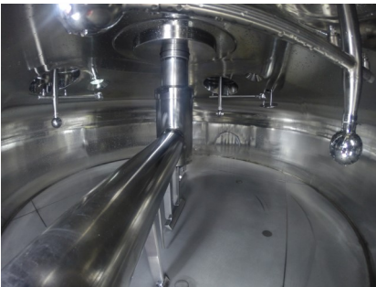
Spray Balls for Cake Washing & CIP
