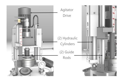
The agitator and the agitator drive, including the gear box, are mounted to a horizontal plate atop the filter vessel. The agitator moves along with this whole assembly which is driven up and down by two hydraulic cylinders. This arrangement allows the agitator to continue rotating while moving up or down. The agitator can be set to cycle up and down on its own can be stopped and held at any desired height.
