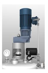
The electric motor can be driven by a VFD providing accurate speed control (usually 0-40 rpm) in either forward or reverse directions. Directional control, combined with an optimized blade design, allows cake smoothing, mixing and discharge.
