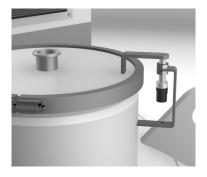
The ZWAG filter can be fitted with proximity sensors to provide open/closed, locked/unlocked positions feedback.
