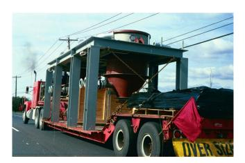
We ship oversize loads via double drop trailers and know the maximum container sizes to avoid oversize load designation. In fact our skidded systems are expressly designed to fit standard over-the-road size requirements.
