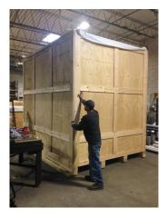
We ship our larger equipment and spare parts in wooden crates designed and built to securely constrain the products. All of the wood we use has been heat treated and is approved for both domestic and world-wide destinations.
